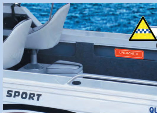
SAFETY EQUIPMENT LOCATION BECOMES OBSCURED WHEN HATCH IS CLOSED
